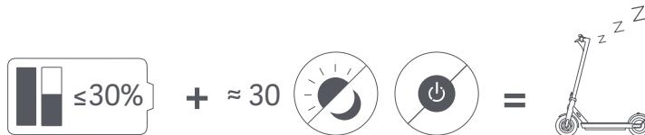
**EN** When the scooter is turned off for about a month with the battery level of the scooter being lower than 30%, the scooter will enter sleep mode. In this case, the scooter cannot be turned on. To exit the sleep mode, charge the scooter for about three seconds to activate the battery.
