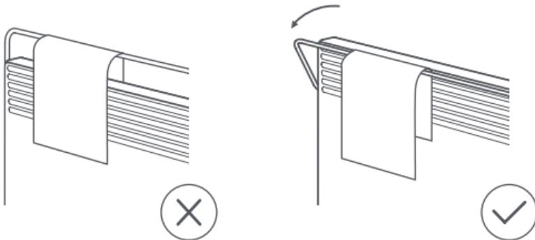
Note: Place the heater on level ground and do not hang a load of more than 1.5 kg on the drying rack.
